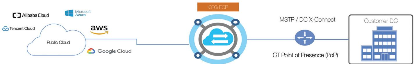
For private cloud environments located in a data center which already has an ECP Point-of-Presence (PoP), a cross connect is required between the ECP PoP to the customer’s rack. For on-prem environments a local MSTP is required to connect to the nearest ECP PoP. Customers use management portal to provision the cloud end connection using either a layer-2 or layer-3 ECP interconnect.
